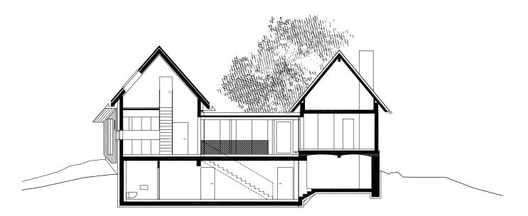
Cross section showing the new house, glazed connecting wing and the old wine cellar building. What is an underground level on the northern edge, is emerging from the hill on the opposide side of the building. At the southern facade, just next to sanitary facilities there is sauna, opening towards a little terrace.
